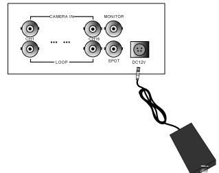
Connect one DC 12V, 6.67 A Adaptor to the back side of Power Jack for right operation of 2HDDs and CDRW.
